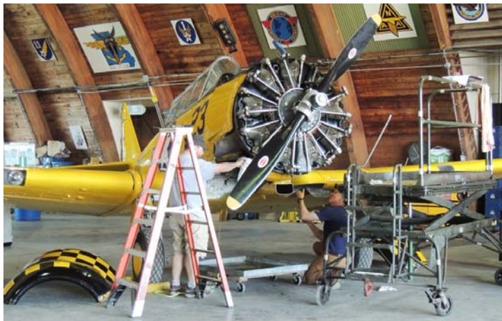
John Fester's T6 getting a new engine cylinder.
